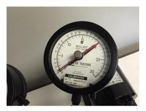
Our gauges scale from 15 to 300 PSI and are precisely calibrated to 0.5% full scale.
