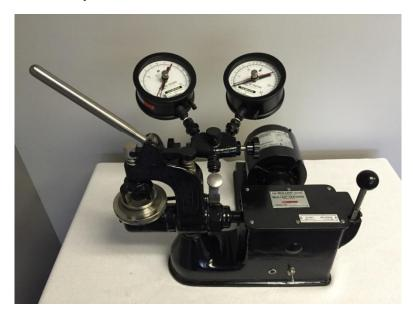
Since its invention in 1887, the Mullen® Burst Tester has been the industry benchmark for measuring the burst strength of paper, paperboard, nonwovens, textiles, plastics and medical materials. Mullen® is cited in many TAPPI, ASTM, INDA and International Standards – and when it comes to quality control, our tester is an integral part of any well-equipped lab.
